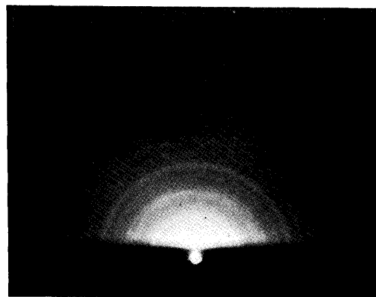
Photo. 7. Diffraction pattern of TiO 2 (anatase and rutile) produced on Ti surface after immersion in boiling 10% CrO 3 -solution for 10 hrs.
