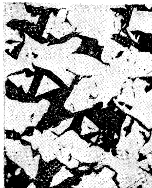
Photo. 2. 5°C below liquidus at eq. state, 20% Sn.
