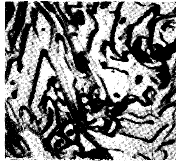
Photo. 64. ×1000 75.07% Mn, 2.46% C; quenched at 700°C in ice brine water; the white part is C ternary solid solution and the gray part \alpha manganese ternary solid solution and the amount of \gamma C ternary solid solution is very small.
