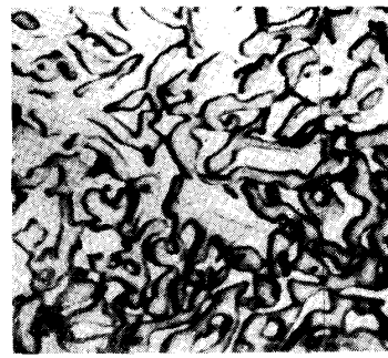
Photo. 62. ×1000 84.75% Mn, 2.40% C; quenched at 700°C in ice brine water; the black part is \gamma C ternary solid solution and the ground mass \alpha manganese solid solution, the eutectoid structure.
