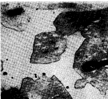
Photo. 36. × 400 89.87% Mn, 0.92%C; quenched at 700°C in ice brine water; \gamma C ternary solid solution and ground mass of \alpha manganese ternary solid solution.
