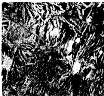
Photo. 21. × 200 74.84%Mn, 4.54%C ; quenched at 1100°C in ice brine water ; \beta C ternary solid solution is martensitic and a small amount of C ternary solid solution is white.
