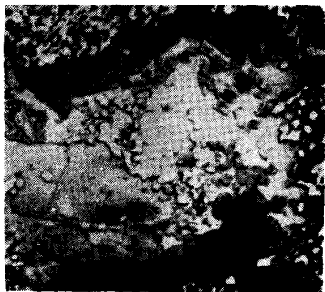
Photo. 37. ×400 71.29 % Mn, 3.17% C; quenched at 1000°C in ice brine water; primary crystal of \gamma manganese ternary solid solution and white part is C ternary solid solution.
