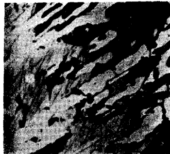
Photo. 46. × 400 70.88 % Mn, 5.61 % C; quenched at 900°C in ice brine water; the black part is \gamma C ternary solid solution, the white part C ternary solid solution and mid-coloured part \gamma manganese ternary solid solution.
