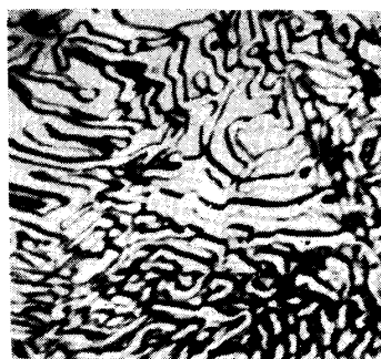
Photo. 60. ×1000 70.52% Mn, 2.07% C; quenched at 700°C in ice brine water; ternary eutectoid structure, the white part is C ternary solid solution, the gray part \alpha manganese ternary solid solution and the black part \gamma iron ternary solid solution.
