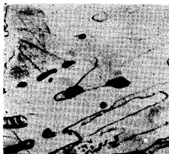
Photo. 47. × 400 70.58 % Mn, 4.92 % C; quenched at 700°C in ice brine water; the black coloured part is \gamma C ternary solid solution and its amount is the least, the white part C ternary solid solution and mid-coloured part \alpha manganese ternary solid solution.
