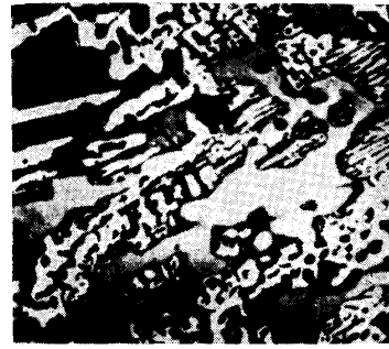
Photo. 4. ×100 63.99%Mn, 3.05%C; slowly cooled from melt; primary crystal of \gamma manganese ternary solid solution and binary eutectic and a small amount of ternary eutectic.
