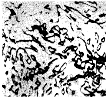
Photo. 61. ×1000 73.25% Mn, 2.26% C; quenched at 700°C in ice brine water; \alpha manganese ternary solid solution and C ternary solid solution and a small amount of \gamma iron ternary solid solution.
