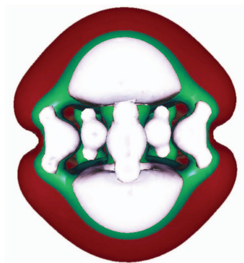
FIG. 8. (Color) \text{Cu}_7 spin density, isosurface coloration: white \rho_s=0.01 e/\text{\AA}^3 , green \rho_s=0.005 e/\text{\AA}^3 , and red \rho_s=0.001 e/\text{\AA}^3 .
