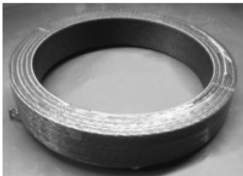
Fig. 4. Dummy coil wound using the 3 + 4 strand cable and impregnated with epoxy resin.
