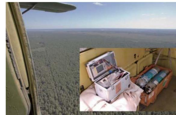
Forest in West Siberia and CO<sub>2</sub> measurement device onboard the aircraft.
