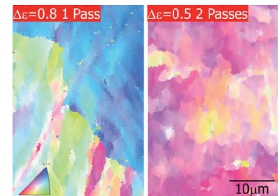
Fig.4 Crystal orientation maps in pure (2N) aluminum after MDF. (a) 1 pass with Δε = 0.8, (b) 2 passes with Δε = 0.5.
