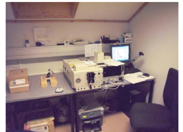
Fig. 7. FTIR instrument in AWI observatory.
