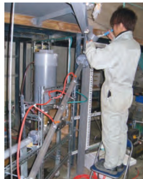
The experimental device to separate soil from crushed asphalt under grizzly, using free fall and spiral flow.
