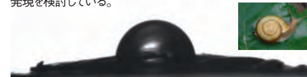
Fig.2 Snail shell doesn't show the superhydrophobic or superhydrophilic surface
