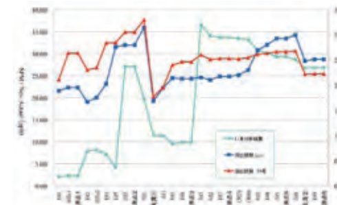
Fig.3 Calculated and measured value of Zn concentration in river water.
