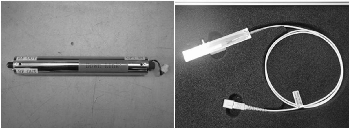
Fig.3.12 Optical link system (a) Down link (Antenna) (b) An optical probe.
