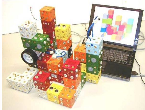
Figure 2.8: ActiveCube: An example of 3D structure with 39 cubes
