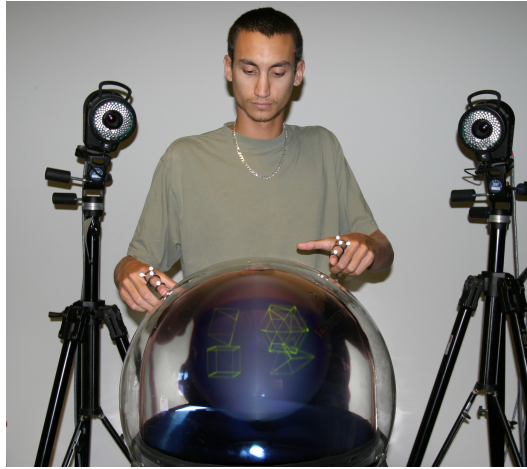
Figure 2.6: Gestural interaction with a volumetric display
