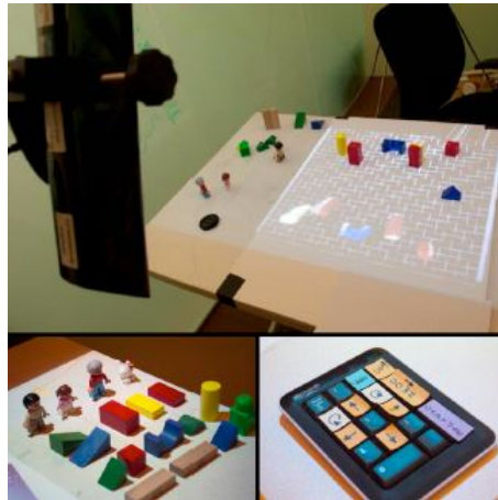
Figure 2.9: StereoBlock: shape recognition based on Kinect
