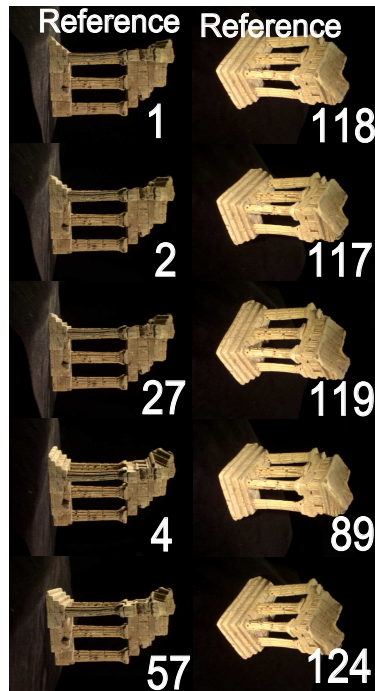
Fig. 3.5 Storage of images in GPU memory, an array row is conformed by the reference view images and the corresponding neighbor views in the rest of columns
