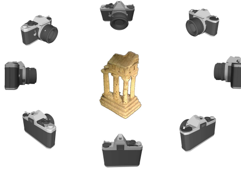
Fig. 2.1 Multi-View Stereo set up, requires multiple images of an object from different view angles
