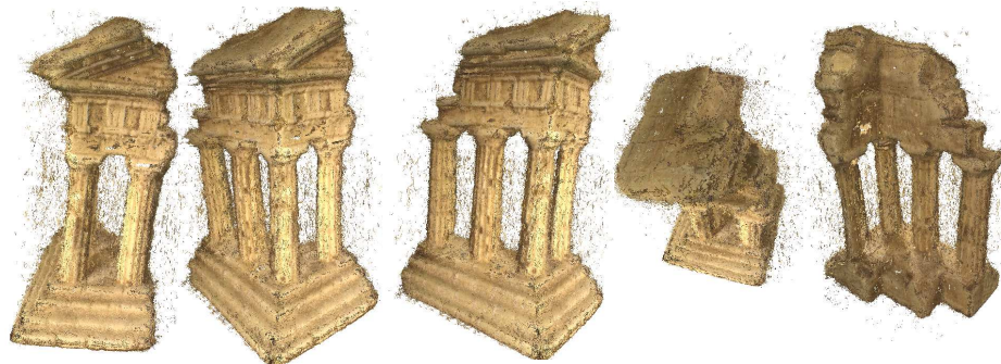
Fig. 4.5 Depth map for whole temple set, five angles of the reconstructed depth map using the original algorithm over all the 312 images of the data set. Rendered with MeshLab [2]
