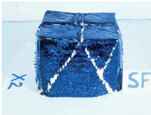
FIG. 1 (color). A dry dense sand cubic specimen ( 100 \times 100 \times 100 \text{ mm}^3 ) that was sheared by a triaxial test apparatus that can control three principal stresses independently. The specimen was surrounded by six rigid planes, and was deformed into a right-angled prism with confining pressure of 300 kPa.
