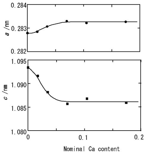
Fig. 3. Lattice parameters ( $a$  and  $c$ ) vs. nominal Ca content in  $\gamma\text{-Na}_{0.70}\text{Ca}_x\text{CoO}_{2-\delta}$  system.
