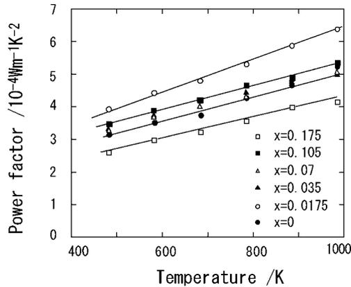
Fig. 6. Temperature variations of power factor of  $\gamma$ - $\text{Na}_{0.70}\text{Ca}_x\text{CoO}_{2-\delta}$ .
