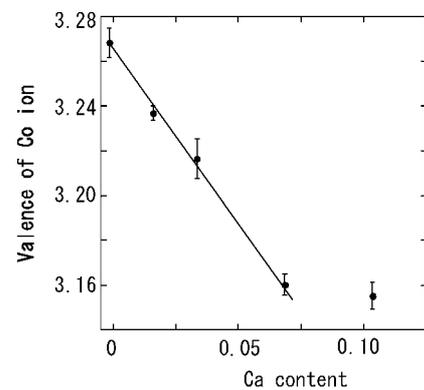
Fig. 4. Valence of Co ion vs. Ca content in  $\gamma\text{-Na}_{0.70}\text{Ca}_x\text{CoO}_{2-\delta}$  system.
