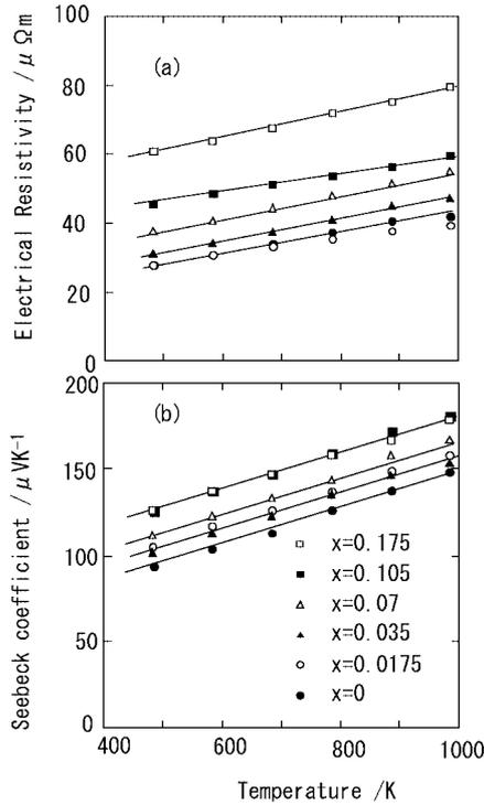
Fig. 5. Temperature variations of electrical resistivity (a) and Seebeck coefficient (b) of  $\gamma$ - $\text{Na}_{0.70}\text{Ca}_x\text{CoO}_{2-\delta}$ .
