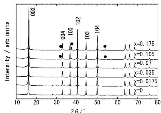
Fig. 1. Powder X-ray diffraction patterns of  $\gamma$ -Na<sub>0.70</sub>Ca<sub>x</sub>CoO<sub>2- $\delta$</sub> . Closed circles indicate the impurity peaks (CaO).
