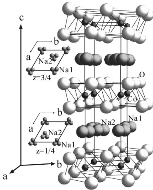
Fig. 2. Crystal structure of  $\gamma\text{-Na}_{0.70}\text{CoO}_2$ . Possible sites in Na sheets at  $z=1/4$  and  $3/4$  are schematically represented. Na(1) and Na(2) ions are statistically distributed over three equivalent positions, respectively. Their sites are not fully occupied with  $\text{Na}^+$ .
