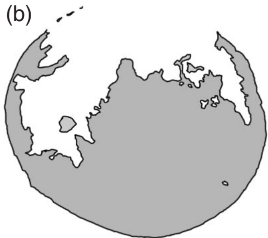
Fig. 4 (a) Scanning electron micrograph of the surface of the OAp-coated specimen after the adherence test and (b) schematic illustration of remaining epoxy glue on the surface.
