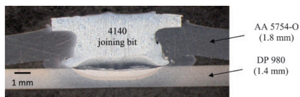
7 Macrocross-section of AA 5754 (top layer) joined to DP 980 (bottom layer): steel 4140 bit was used in joining process
