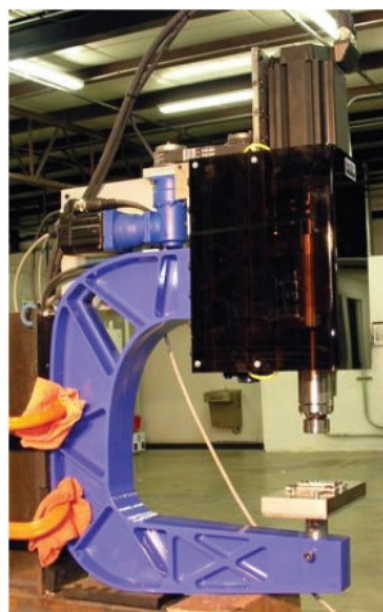
2 C frame welding machine used for FBJ experiments
