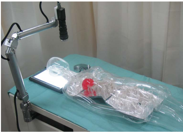
Fig.17 Surgical simulator for endovascular neurosurgery, which allow evaluating stress condition on arterial structure applied with surgical operation and blood streaming, using photoelastic modality
