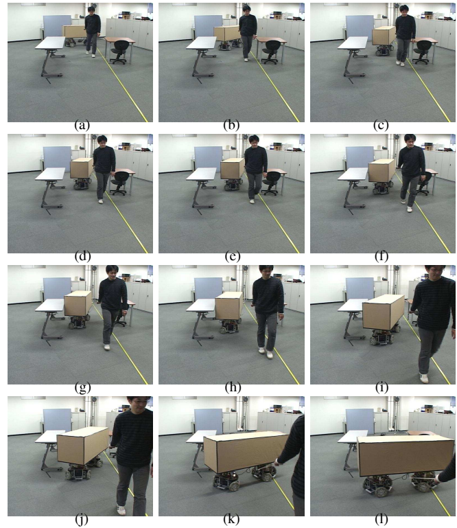
Fig. 12. Orientation Control for Passing an Object through a Narrow Place: Only the pulling force is applied to the center of the object-robot system. PRPs rotate the object to an orientation cooperatively when they are passing the narrow place, and more the object back to the initial orientation finally.
