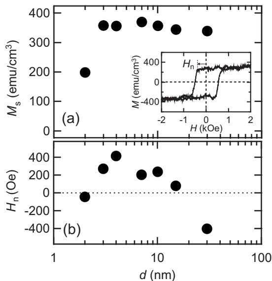
FIG. 2. Dependence of (a) saturation magnetization  $M_s$  and (b) nucleation field  $H_n$  on the CoCrPt film thickness. The inset shows magnetization curves for the  $4\text{-nm}$ -thick CoCrPt film.
