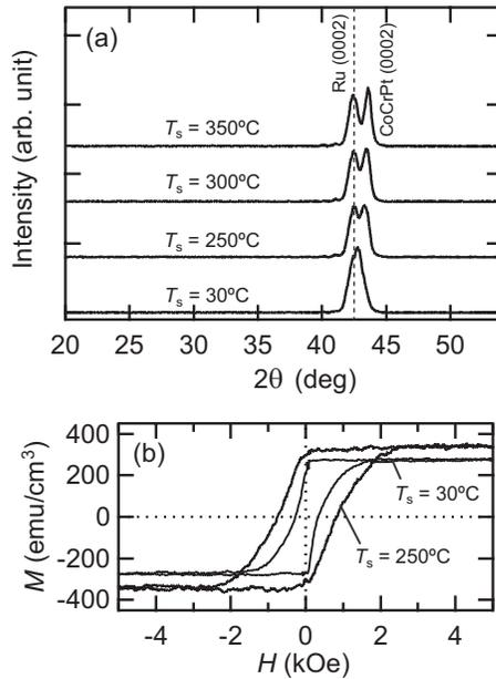
FIG. 1. (a) XRD profiles of Ta/Ru/CoCrPt/Ta structures. The CoCrPt films were deposited at  $T_s=30, 250, 300,$  and  $350$  °C. (b) Magnetization curves with applied field perpendicular to the plane for CoCrPt films deposited at  $T_s=30$  and  $250$  °C.
