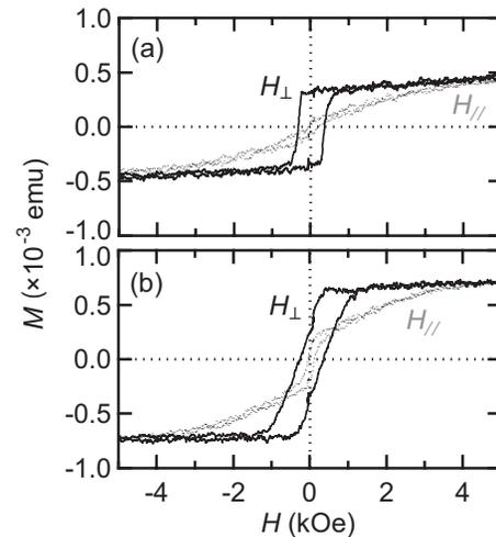
FIG. 3. Magnetization curves for the stacking of (a) CoCrPt/CoFe/Ru/CoFe (bottom electrode) and (b) CoFe/Ru/Co/CoCrPt (top electrode) in the perpendicularly magnetized MTJs. Magnetic fields were applied both perpendicular ( $H_{\perp}$ ) and parallel ( $H_{\parallel}$ ) to the film plane.
