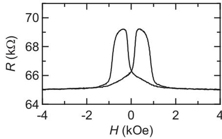
FIG. 4. Typical TMR curve for the MTJ with a synthetic ferrimagnetlike structure using perpendicularly magnetized CoCrPt layers.
