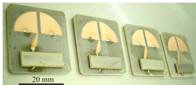
Figure 1. Developed 2.45 GHz wireless temperature transponders, consisting of packaged SAW delay line sensors mounted on a microstrip antenna.
