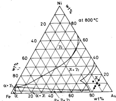
Fig. 1. Phase diagram of Au-Fe-Ni system at 800°C (after Köster *et al.* [2]). Studied alloys are shown by solid circle.
