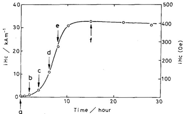
Fig. 7. Intrinsic coercive force of Au-10% Fe-10% Ni alloy aged at 400°C.
