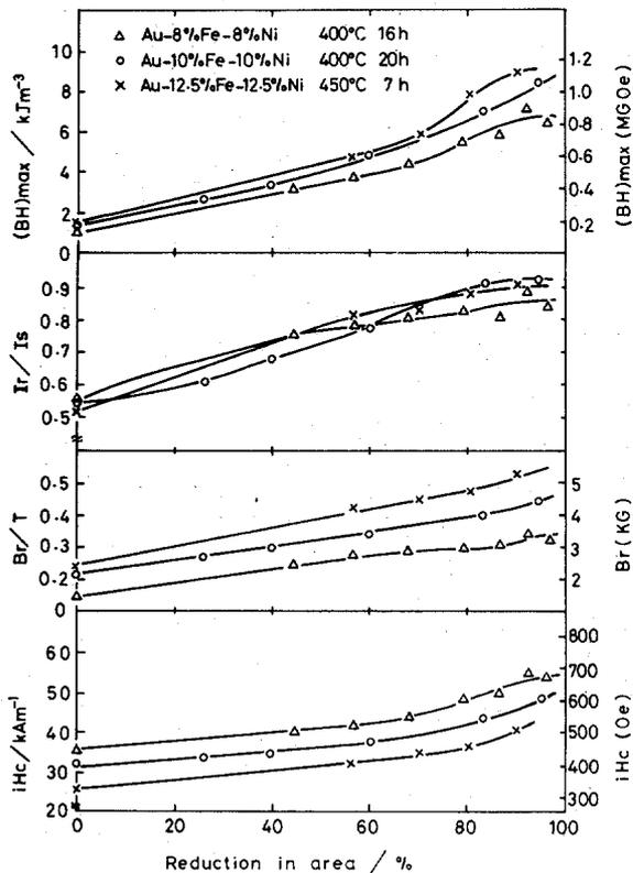
Fig. 5. Effect of cold-swaging on magnetic properties of Au-Fe-Ni alloys.
