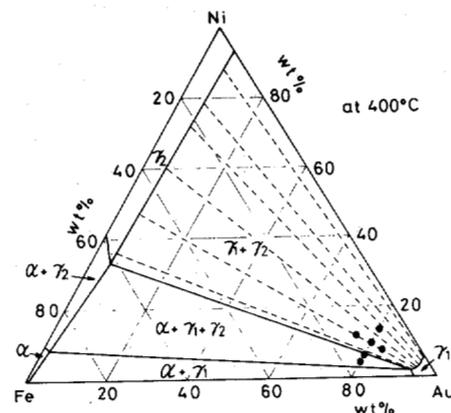
Fig. 2. Phase diagram of Au-Fe-Ni system at 400°C (after Köster *et al.* [2]). Studied alloys are shown by solid circle.
