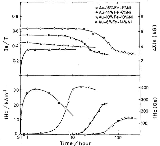
Fig. 4. Intrinsic coercive force  $iH_c$  and magnetization intensity  $I_s$  of Au-Fe-Ni alloys after aging at 400°C.
