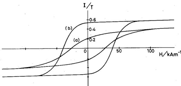
Fig. 6. Magnetization curves of Au-12.5% Fe-12.5% Ni alloy. (a) Before swaged. (b) After swaged, 92 percent reduction in area.
