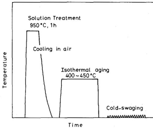
Fig. 3. Schematic diagram of heat treatment and cold-swaging.
