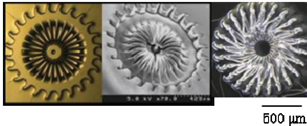
Fig. 11 Complicated 3D patterning of KMPPR
