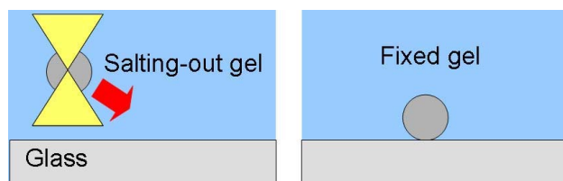
Fig. 7 A schematic of fixing gel on the glass plate
