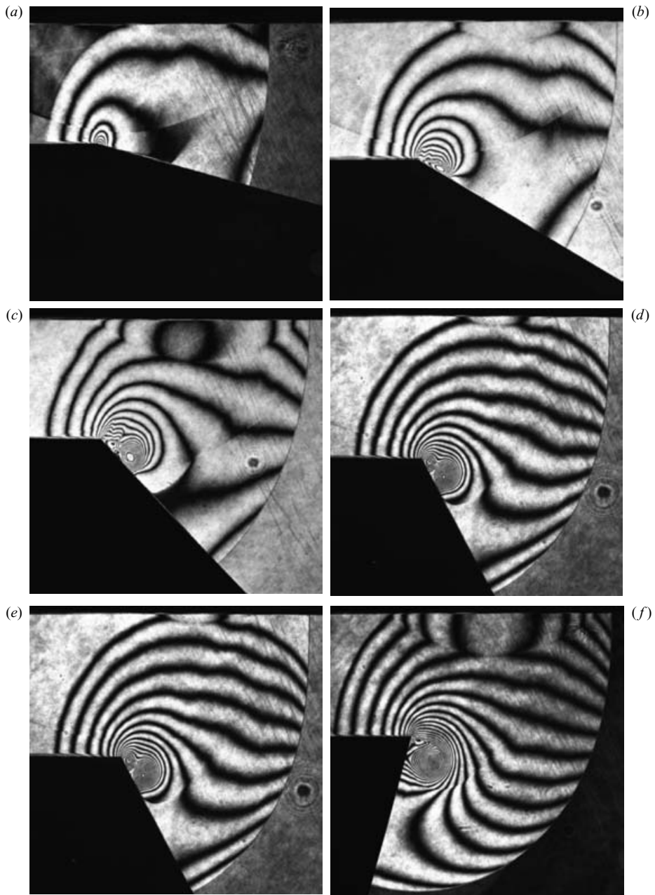
FIGURE 6. Results of shock diffraction in nitrogen taken by holographic interferometry: (a) \theta = 15^\circ , M_s = 1.51 ; (b) \theta = 30^\circ , M_s = 1.50 ; (c) \theta = 45^\circ , M_s = 1.50 ; (d) \theta = 60^\circ , M_s = 1.40 ; (e) \theta = 90^\circ , M_s = 1.40 ; (f) \theta = 105^\circ , M_s = 1.40 .
