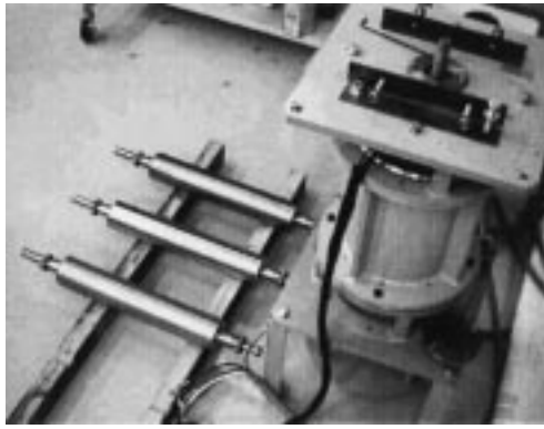
Fig. 6. Cylindrical secondary conductors of solid metals.
