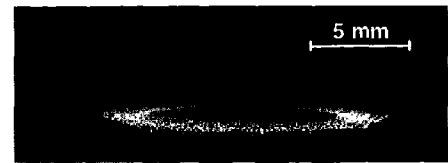
Fig. 6. (a) Radial profiles of floating potential V_f . Dotted curve corresponds to V_c = V_{r,1} = -20 V and V_{r,2} = -50 V. Solid curve corresponds to V_c = V_{r,2} = -50 V and V_{r,1} = -20 V. (b) CCD image of a ring-typed fine-particle cloud.
