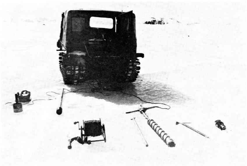
Photo 7 Equipment for echo-sounding; sander, pickel, core drill, wire for plummet and tranceducers from right to left.
