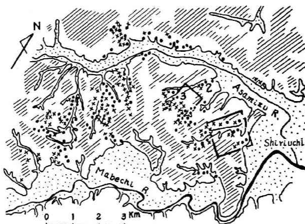
Fig. 3 Failed zones in the region to the west of Hachinohe spot: failed zone with Scauper-type erosion area, cross: failed zone with Plane-type erosion area, hatch: upland surface, blank: valley wall, stipple: valley floor and the lowest terrace Encircled areas with heavy lines are shown in Fig. 4.
