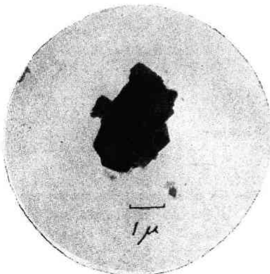
Fig. 27 A fog nucleus in Sendai under intense bombardment, presumed to be a soil particle.
