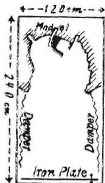
Fig. 3 Model of Shizukawa Bay in the Tank. The blackened area indicates breakwaters built after 1933.
