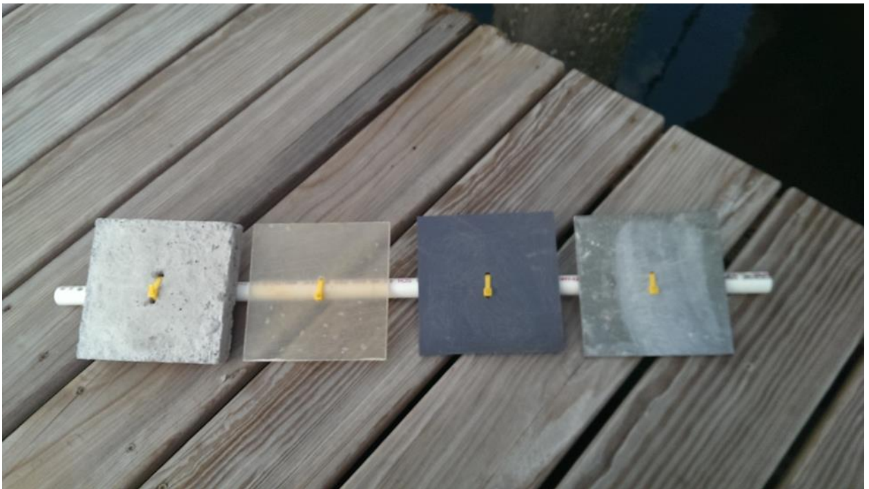
Figure 1. General set up of a set of four 14x14cm fouling plates attached to a PVC pipe with zip ties. Order of plates from left to right: Concrete, Fiberglass, PVC, and Slate.
