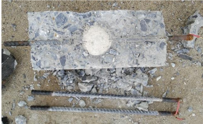
Fig. 23. Reinforcing steel of prism specimen after 180 days of exposure to chlorides.
