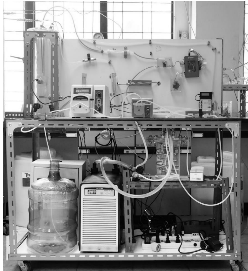
Fig. 1. An experimental unit of a basic wastewater neutralization by carbon dioxide.
