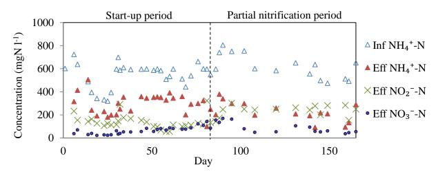
Fig. 1. Performance an entrapped cell-based partial nitrification reactor.
