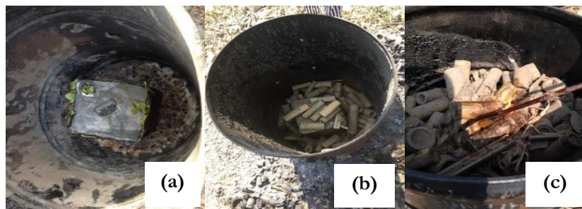
Fig. 2. (a) Raw materials were packed in a 10-L bucket; (b) The 10-L bucket with raw materials was put in a 200-L tank; (c) Bamboo was filled in the 200-L tank as fuel, and it was fired using diesel oil.
