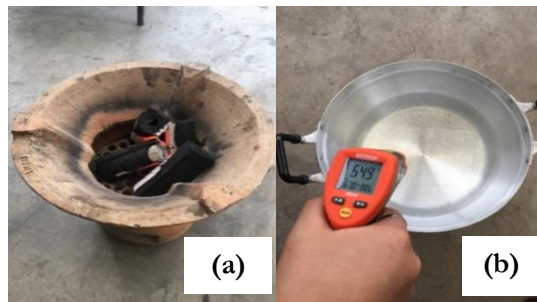
Fig. 14. (a) A fire is set on the carbonized briquette on a stove; (b) The water temperature is recorded using Extech Infrared Thermometer 42512.
