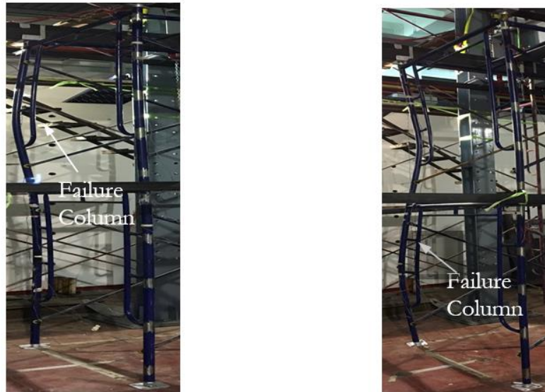
a) Single-Curvature Buckling (specimen S2D0-1) b) Double-Curvature Buckling (specimen S2D1-3)
