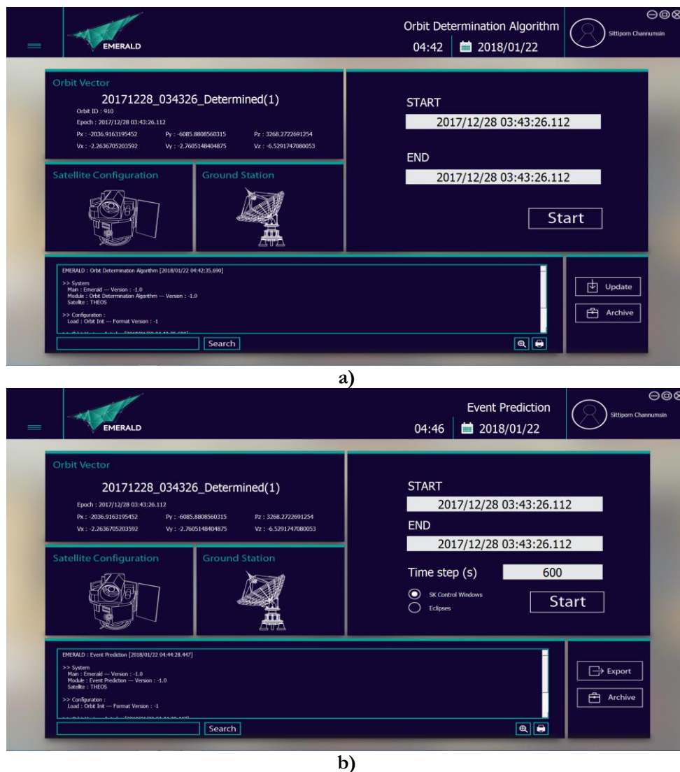
Fig. 20. GUI a) orbit determination b) event prediction.
