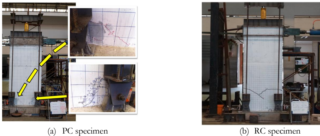
Fig. 14. Crack development in specimen.
