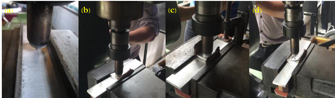
Fig. 2. The friction stir spot welding process.
