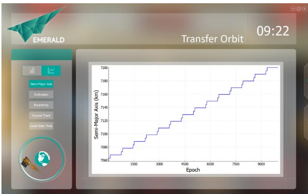
Fig. 12. Transfer orbit GUI a) transfer orbit input b) semi-major axis evolution after 14 maneuvers.
