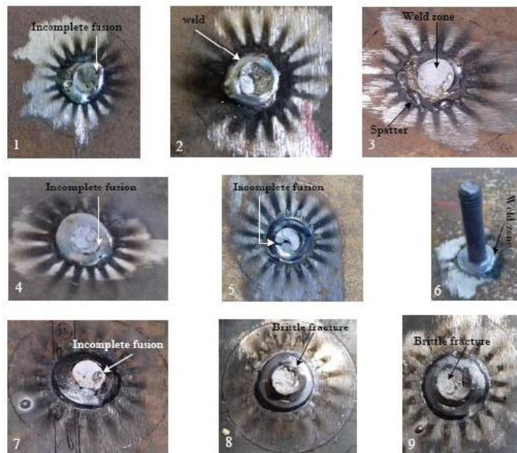
Fig. 9. The fractured specimens by torsional test.
