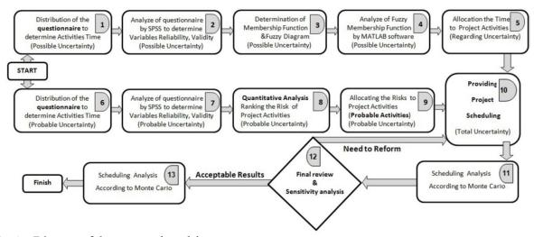
Fig. 6. Diagram of the proposed model.
