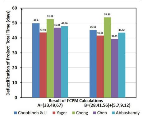
Fig. 5. Results of project time calculation by various fuzzy ranking methods.
