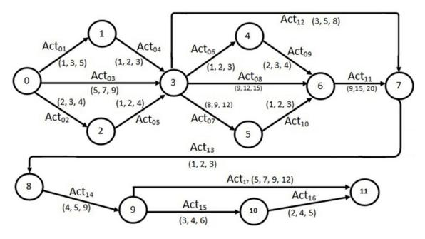
Fig. 3. CPM of the nitrogen package project by fuzzy approach.
