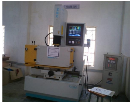
b. Electric discharge machine used for machining of Micro-grooves on the rake face of WC cutting tools
