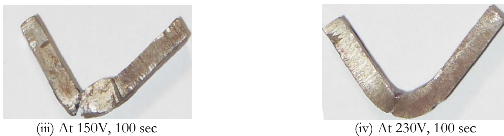
Fig. 5. (b) Specimens after impact failure.
