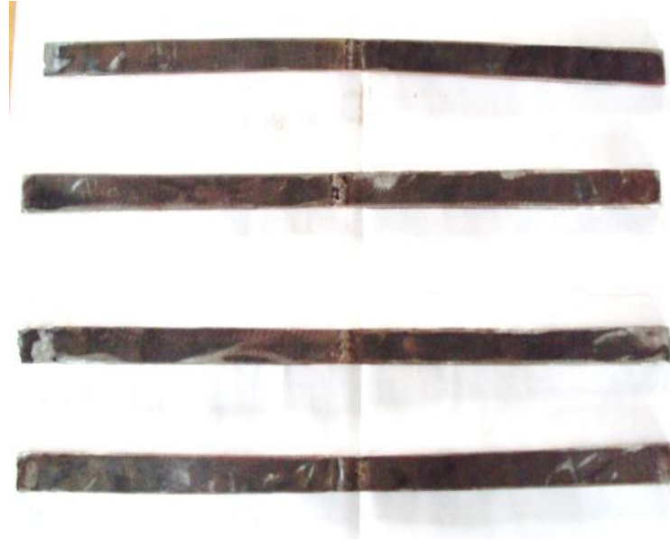
Fig. 3. (a) Produced specimens for Flexural test.
