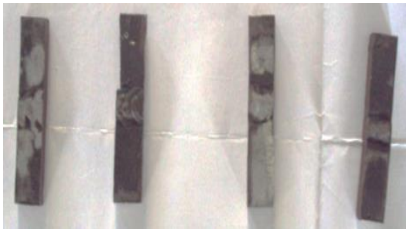
Fig. 5. (a) Specimen samples prepared at different vibration parameters for impact test.
