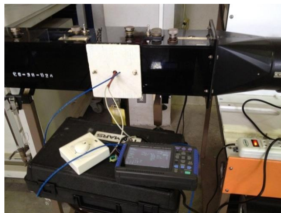
Fig. 4. The testing section with a heater installing and temperature recording by the data logger through the K-type thermocouple wire.
