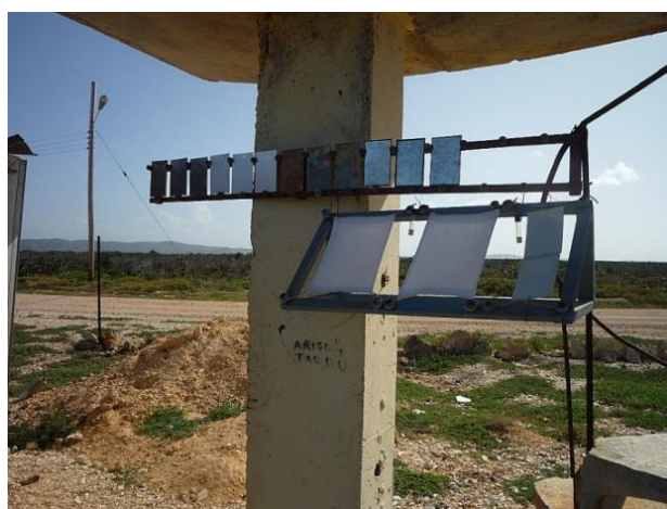
Fig. 2. Outdoor exposure sites with four atmospheric pollutants devices and three specimens of four metals: carbon steel, aluminum, copper and galvanized steel placed in the wooden racks.
