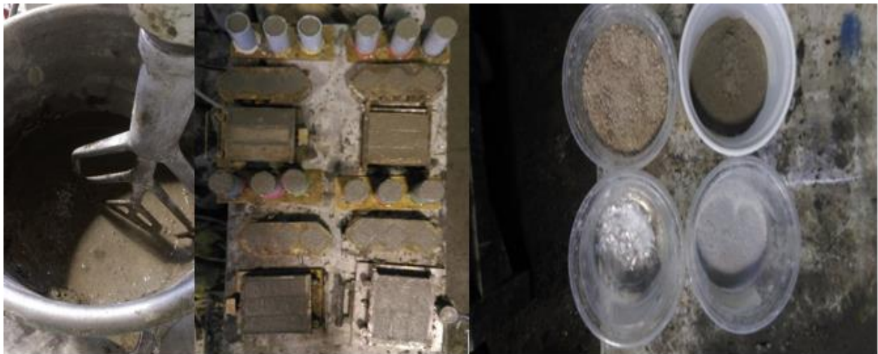
Fig. 2. The used materials, the samples casted in the molds and the method of mixing the materials.
