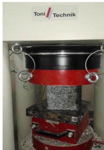
Fig. 3. Apparatus of measuring compressive strength.
