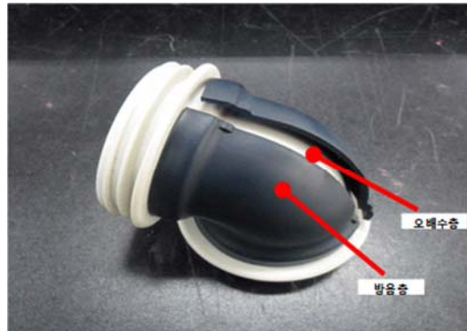
Fig. 5. A pipe fitting outer layer made by post-consumer CC compound.
