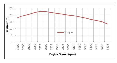
Fig. 5. Engine torque curve.
