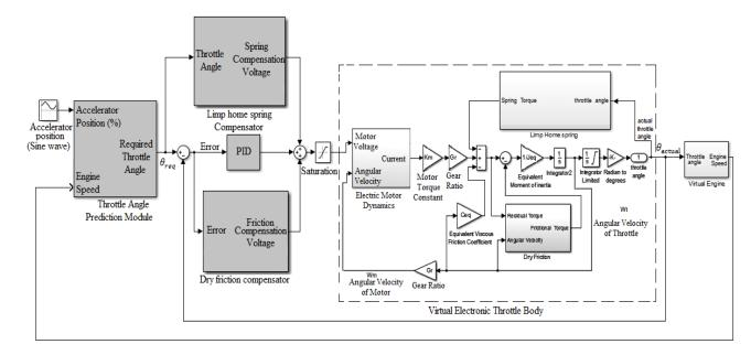
Fig. 9. Schematic of the proposed electronic throttle control system.
