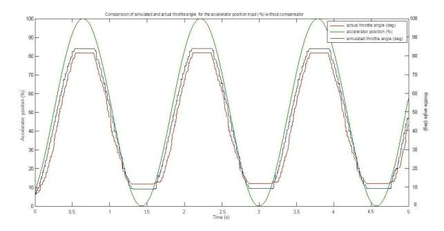
Fig. 14(a). Simulated and actual throttle angle for accelerator position input without compensators for sine input.
