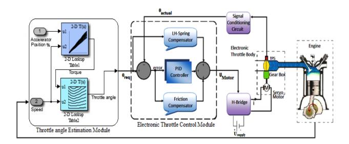
Fig. 4. Proposed schematic of electronic throttle control system.
