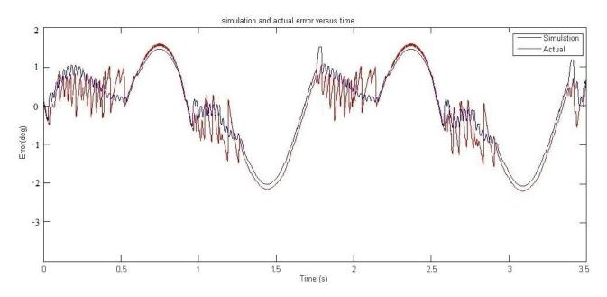
Fig. 13(b).Comparison of throttle angle error with compensator for sine input.
