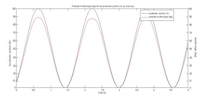
Fig. 12. Estimated throttle angle ( $\Theta_{req}$ ) from throttle estimation module for accelerator position sine input.
