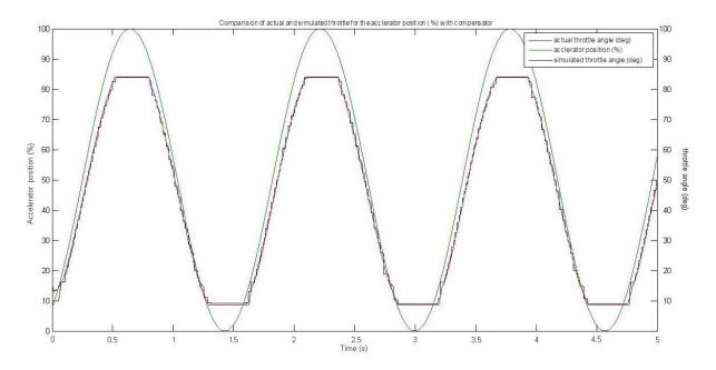
Fig. 13(a). Simulated and actual throttle angle for accelerator position input without compensators for sine input.
