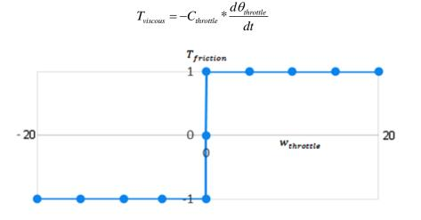
Fig. 3. Variation of frictional torque with throttle angular velocity.
