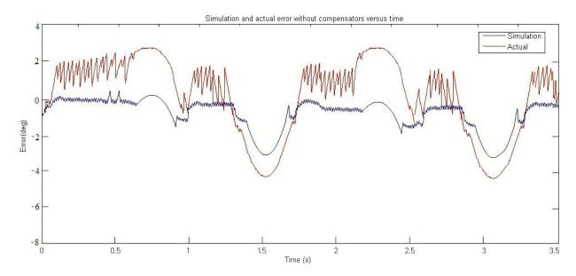
Fig. 14(b). Comparison of throttle angle error without compensator for sine input.
