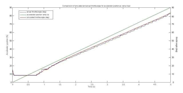
Fig. 15. Simulated and actual throttle angle for accelerator position input with compensators for ramp input.
