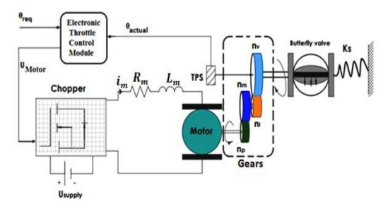
Fig. 1. Schematic of electronic throttle body system components.
