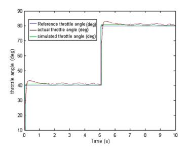
Fig. 11. Simulated throttle angle response for the estimated parameters.
