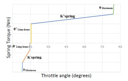
Fig. 2. Variation of spring torque with the throttle angle.
