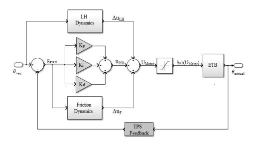
Fig. 8. Electronic throttle body control system module with compensators.
