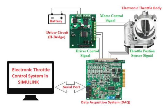
Fig. 10. Schematic of Hardware in Loop (HIL) simulation of electronic throttle control.
