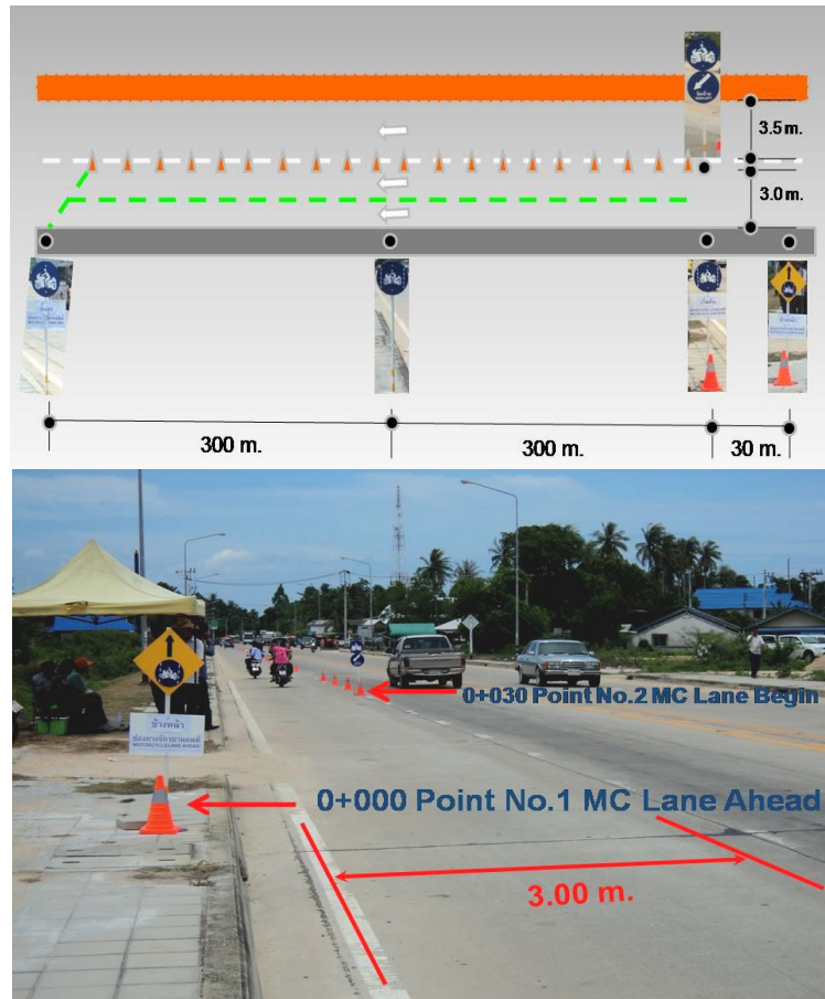
Fig. 3. Field test of MC lane configurations on an urban road in Narathiwat.
