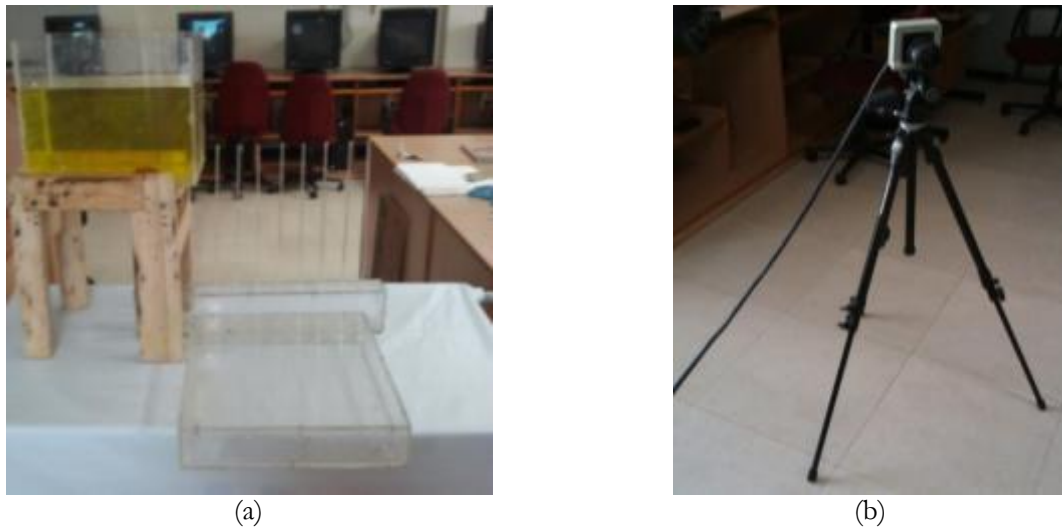
Fig. 12. Experimental set up for flow visualization.
