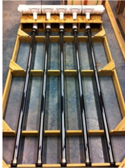
Fig. 8. A solar water heating system with five single ended evacuated solar thermal collectors.
